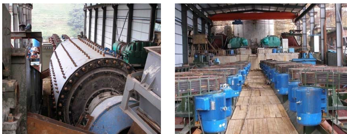
Figure 3: Ball Grinder and Flotation Mill at Damajianshan Mine Beneficiation Plant
